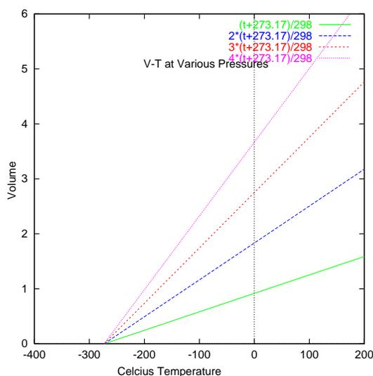
Figure 2: Volume Changes with Temperature
