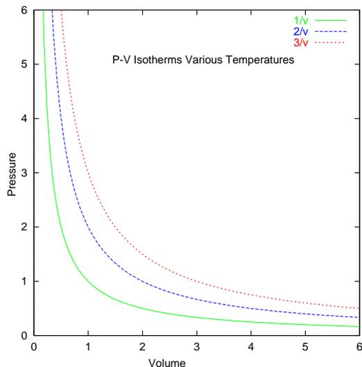
Figure 1: Absolute Pressure - Volume relations at Constant Temperature
